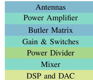
Figure 9. Envisioned structure of the transmitter components in a chip stack. Different background colors indicate different technologies.
