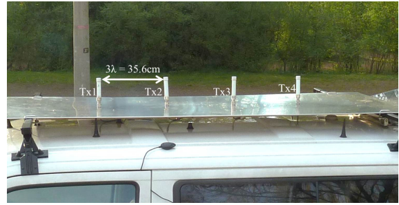
Fig. 2. Configuration of moving relay antennas on measurement bus. Metal plate is used to get homogeneous ground plane below the antennas
