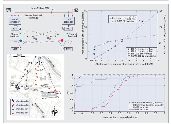
Figure 6. Top left: Distributed implementation of Joint transmission COMP. Top right: Performance and backhaul traffic vs. cluster size obtained from system-level simulations. Bottom left: Intra- and inter-site test scenarios in Berlin [5]. Bottom right: Measured throughput with full frequency reuse in a two-cell scenario w/o external interference relative to the case of isolated cells.
