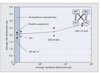
Figure 3. Achieved rates vs. required backhaul for different uplink cooperation schemes, as measured in field trials.
