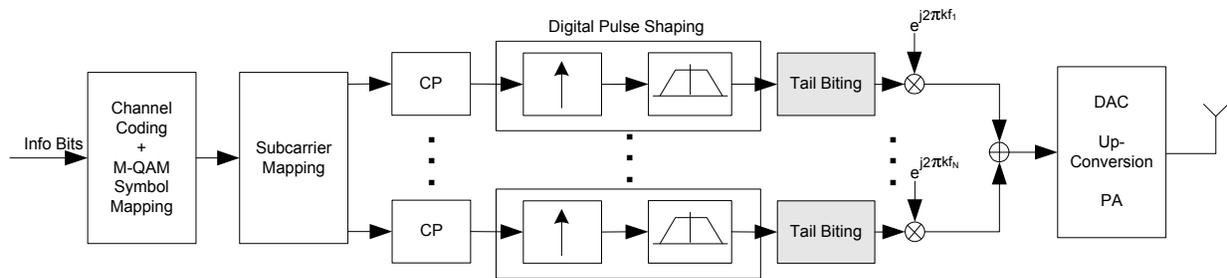
Fig. 1. Principle of the GFDM digital transmitter
