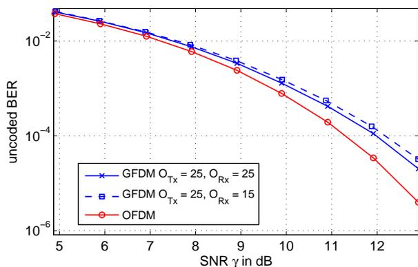
Fig. 5. Bit error rate performance for QPSK modulation, AWGN channel used
