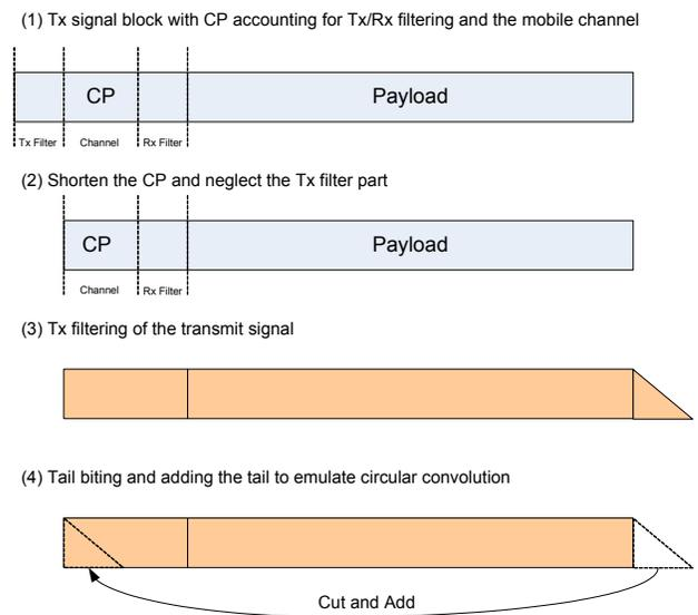
Fig. 3. Principle of CP shortening by tail biting
