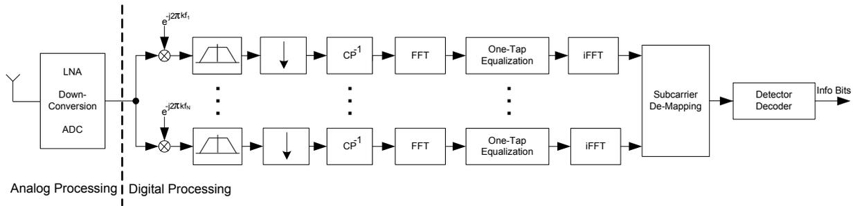
Fig. 4. Principle of the GFDM digital receiver
