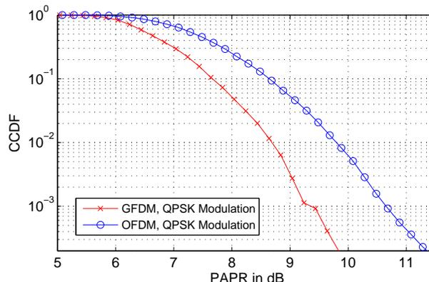
Fig. 6. CCDF of PAPR for GFDM and OFDM
