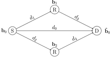
Fig. 1: Lossy forwarding two-relaying system model.
