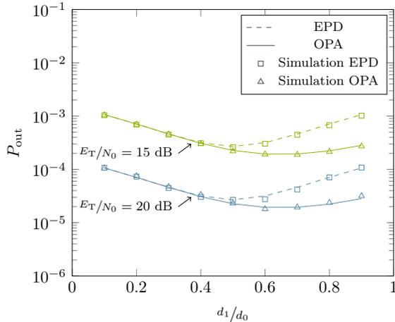
Fig. 6: OP for LFOR system with OPA and EPD at  $E_T/N_0 = 15$  dB and  $E_T/N_0 = 20$  dB.
