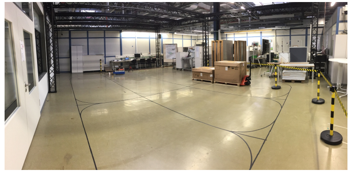
Fig. 1: The size of the surrounding area in which the measurement environment is integrated is about 12\text{ m} \times 22\text{ m} . The available test area itself has a size of 11\text{ m} \times 8\text{ m} .
