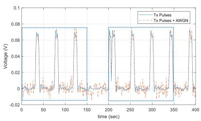
spike generation as well as noise on the wireless channel. As shown in the figure, jitter can cause a temporal shift of pulses, erasure of pulses, or insertion of pulses. This noise and jitter can severely affect the communication performance. In this thesis, the aim is to study the impact of such noise effects on the achievable data rate of spike-based communications.
